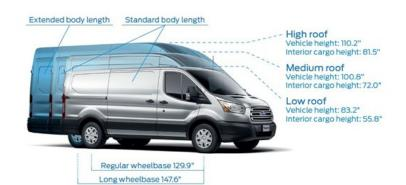
The Transit is available in three body lengths and three roof heights, Nor-Cal Vans primarily works with Medium and High roof Transits.
