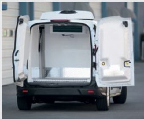
Vanco van liners are built of prefabricated panels so they can be removed to repair collision damages.
